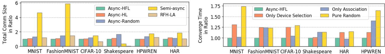
**Figure 7: Left: Total communicated data size in ratio compared to *Async-HFL* on large-scale simulations and various datasets. Right: Convergence time in ratio compared to *Async-HFL* using various combinations of device selection and device-gateway association.**
