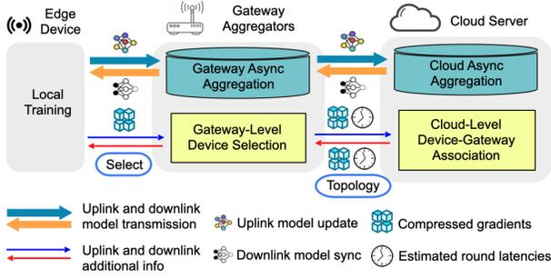
**Figure 6: The overview of the distributed design of gateway-level device selection and cloud-level device-gateway association. The thick arrows represent necessary communications for FL while the thin arrows stand for communication overhead.**
